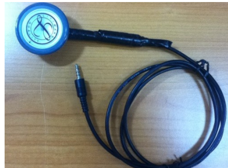
Figure 12. The photo of the Heart Sounds sensor node.
