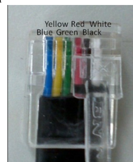
Fig.20 LEGO transmission line header
