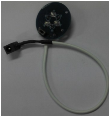
Figure 6. The infrared LED lamp board's physical map
