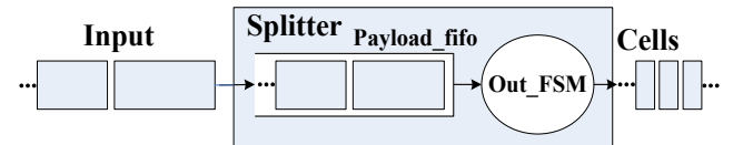
Fig. 7 the design of sub-module Splitter
