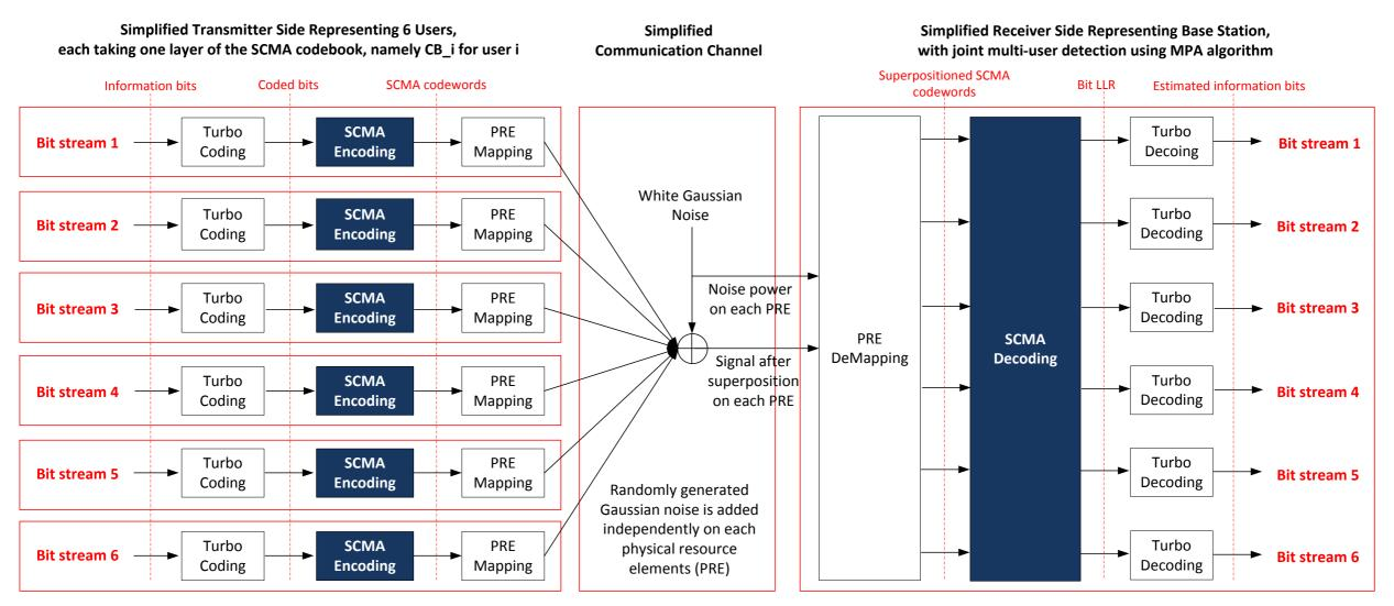
\* Turbo coding and decoding can be replaced by other forward error correction (FEC) channel coding/decoding modules.
